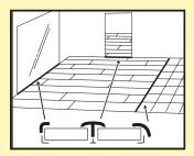
Make sure the subfloor is completely flat. Cement joints between tiles or other gaps of more than 1 mm (0,04inch) in depth and 4 mm (0,16inch) in width should be levelled .
