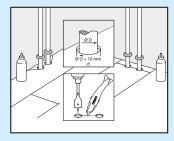
Then, using an appropriate glue along the cut edges of the piece you cut out, glue the piece in place. Be sure no glue comes between the cut out piece and the subfloor.
